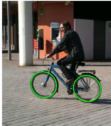
Figure 1.2: The green ellipses indicate measurements obtained from the two bike wheels. The ellipse parameters are later fed through a particle filter framework in order to estimate the bicycle state.
